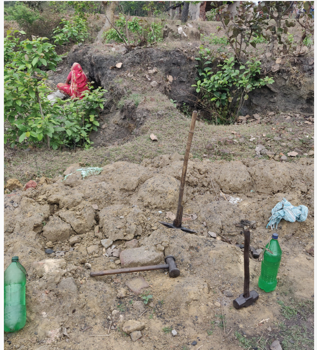
Photo 14: Crudely made tools used by locals when fetching coal to dig out and break chunks of coal
